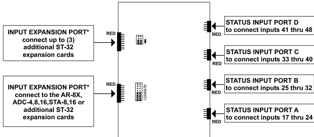
NOTE: The shunt settings shown above are set for inputs 17 thru 48 (ports 3 thru 6). Inputs 1 thru 16 are used for the STA-16 (ports 1 and 2). Connect all ribbon cables with the notch on the ribbon cable connector pointing up. The red conductor should be positioned as shown above.
