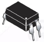
SPST Miniature Solid State Relay 4 amp (1-Form-A) 24 volts DC (rated 2 amp\* above 12 volts) Replaces Optocoupler to provide high current MOSFET output (DC only) Isolation Voltage: 2,500 Vrms (min)
