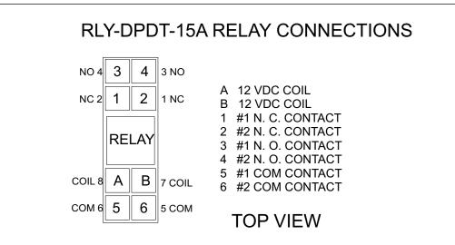
IMPORTANT NOTE: Connect HVAC equipment up to the N. C. contacts so equipment will operate with the relay in a de-energized state.
