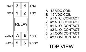
IMPORTANT NOTE: Connect HVAC equipment up to the N. C. contacts so equipment will operate with the relay in a de-energized state.
