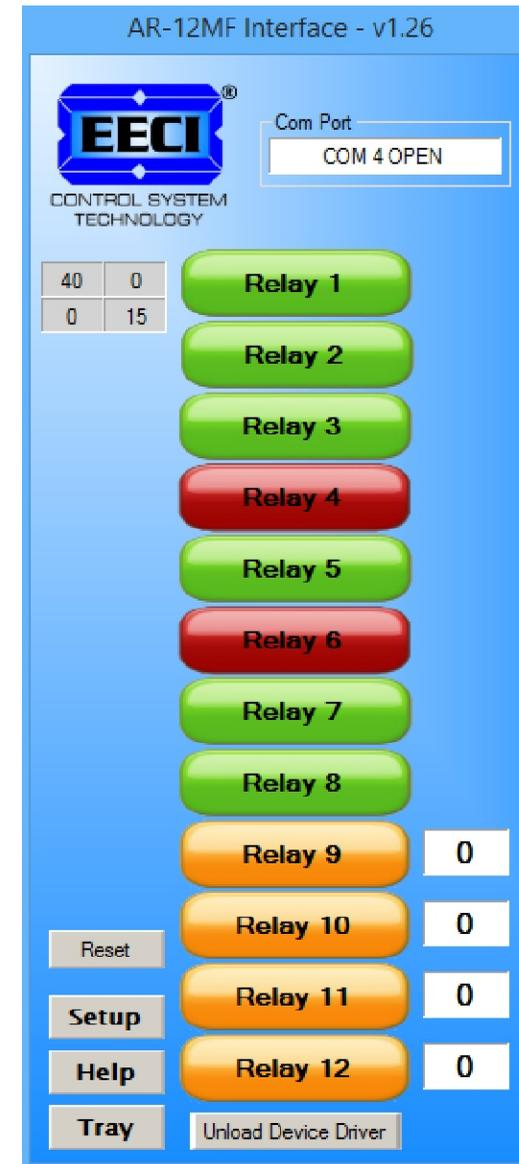
The AR-12MF User Interface allows you to set all of the basic operating characteristics of the hardware and permits the AR-12MF to send and receive data from other Windows applications or programs that you create.
