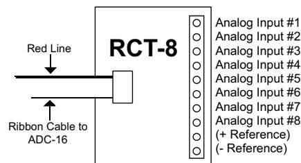
additional testing is desired, connect a 10k ohm 20 turn potentiometer to each input (one at a time) as shown on page 12, figure B. The input shown on the screen should increment from 0 to 255 (8 bit) or 0 to 1023 (10 bit). The number shown for each input should increment by one (in 256 increments for 8 bit inputs) or (in 1024 increments for 10 bit inputs) as the potentiometer is slowly adjusted from 0 to 20 turns.
