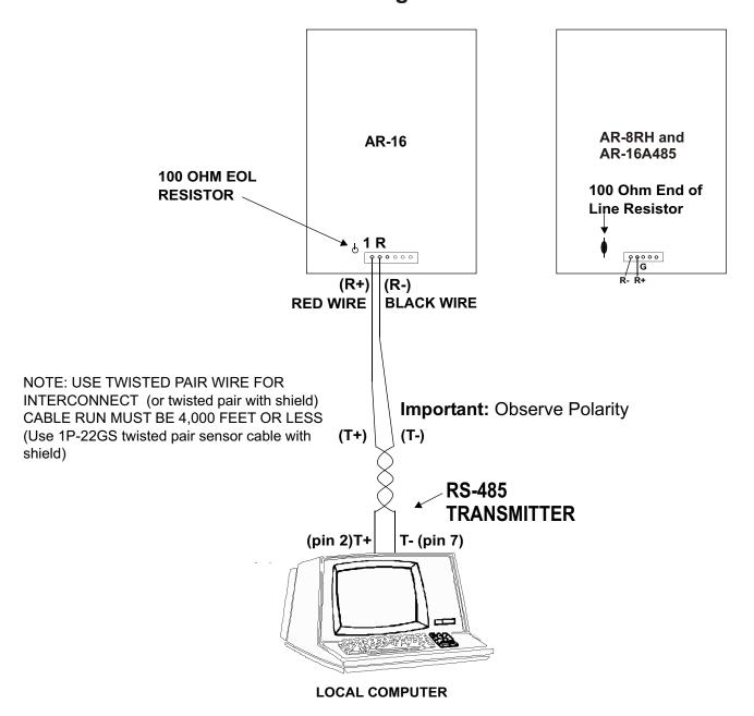
NOTE: The use of shielding on the RS-485 interconnect cable is strongly recommended to protect the RS-485 receiver/driver ICs from damage which may be caused by electrical storm and lightning transients. The shield of the cable should be connected to an earth ground or an equipment ground (connected to your electric system ground via the third prong on the electric cord or connected to a ground rod).
