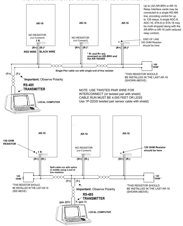
NOTE: The use of shielding on the RS-485 interconnect cable is strongly recommended to protect the RS-485 receiver/driver ICs from damage which may be caused by electrical storm and lightning transients. The shield of the cable should be connected to an earth ground or an equipment ground (connected to your electric system ground via the third prong on the electric cord or ground rod).
