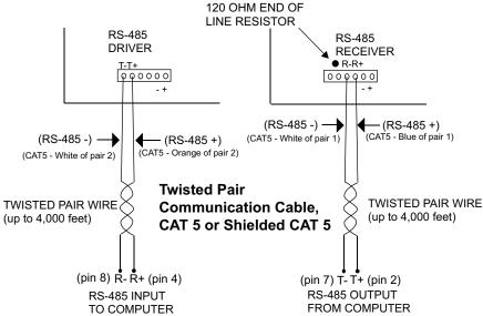
NOTE: The use of shielding on the RS-485 interconnect cable is strongly recommended to protect the RS-485 receiver/driver ICs from damage which may be caused by electrical storm and lightning transients. The shield of the cable should be connected to an earth ground or an equipment ground (connected to your electric system ground via the third prong on the electric cord).
