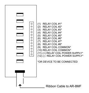
One side of the relay coil of each relay must be connected to one of the relay common terminals (two terminals are provided for all eight relays, terminal #9 and terminal #10).
