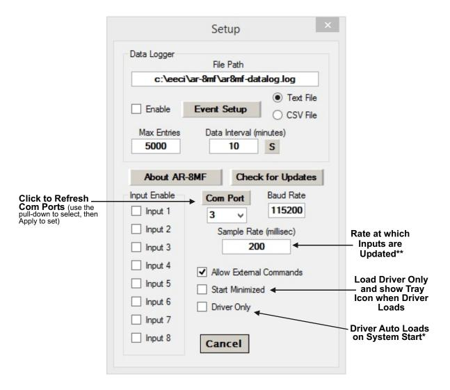
Start the data logger by checking the Enable box. The logger will roll-over or stop based on the setting in the Max Entries box. The Data Interval may be set to minutes or seconds and will log the data based on the setting in the box.
