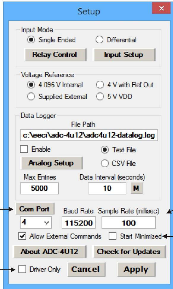
Start the data logger by checking the Enable box. The logger will roll-over or stop based on the setting in the Max Entries box. The Data Interval may be set to minutes or seconds and will log the data based on the setting in the box.
