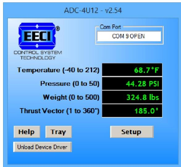
The ADC-4U User Interface allows you to set all of the basic operating characteristics of the hardware and permits the ADC-4U to send and receive data from other Windows applications or programs that you create.
