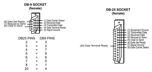
SHOWN ABOVE ARE COMMON CONNECTORS USED FOR CONNECTION TO MOST RS-232 PORTS (the connectors are viewed from the rear/solder side)
