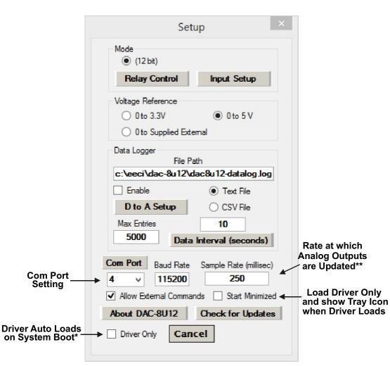
Click the Com Port Button to update the detected com ports in the pull-down. Click the Data Interval Button to toggle between minutes and seconds.
