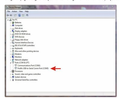
Port" entry, this is your USB Com driver\* and the com port assigned is to the right of the entry. Right click on the entry and select "Properties"and click the "Driver" tab. Your USB Com driver must be Prolific version 3.4.62.293 or higher (dated 10/17/2013 or later). If your USB Com driver is not up to date, right click on the entry and select "Update Driver Software". If your USB Com driver is up to date then please note the Com port number assigned and jump to step 5.
