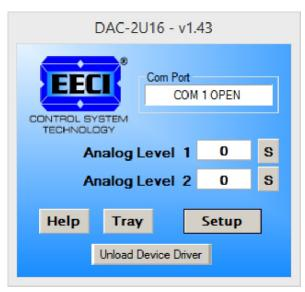
The DAC-2U User Interface allows you to set all of the basic operating characteristics of the hardware and permits the DAC-2U to send and receive data from other Windows applications or programs that you create.
