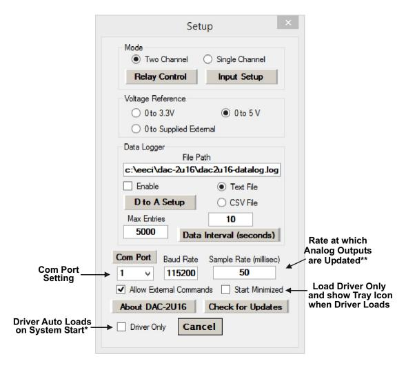
Click the Com Port Button to update the detected com ports in the pull-down. Click the Data Interval Button to toggle between minutes and seconds.
