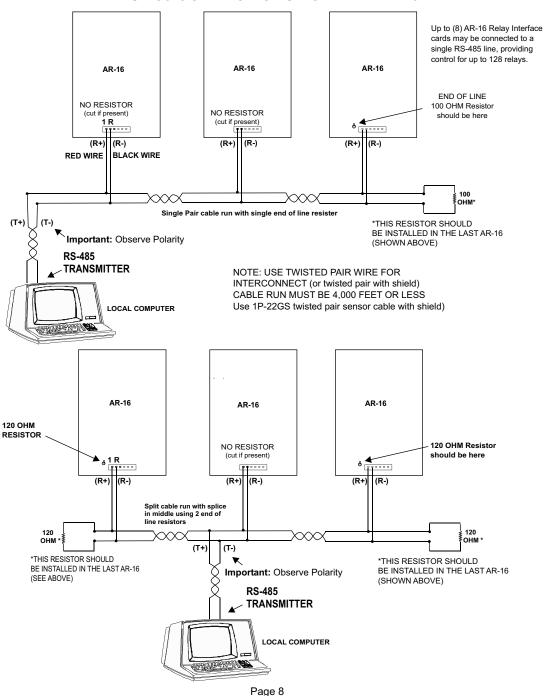
NOTE: The use of shielding on the RS-485 interconnect cable is strongly recommended to protect the RS-485 receiver/driver ICs from damage which may be caused by electrical storm and lightning transients. The shield of the cable should be connected to an earth ground or an equipment ground (connected to your electric system ground via the third prong on the electric cord or ground rod).
