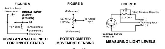
Shown below in figures A, B & C are methods for reading contact closure, potentiometer movement & light levels.
