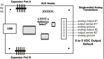
\*after testing is complete (and for best precision) remove the jumper to the analog output terminal and connect the output sense as close as practical to your measurement device. This feature corrects for any voltage drop.
